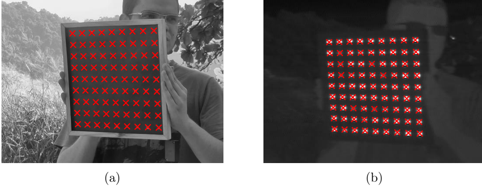
Figure 6.6: Results of the calibration point detection for the (a) visible-light and (b) IR calibration images of Fig. 6.4 (zoomed version).
