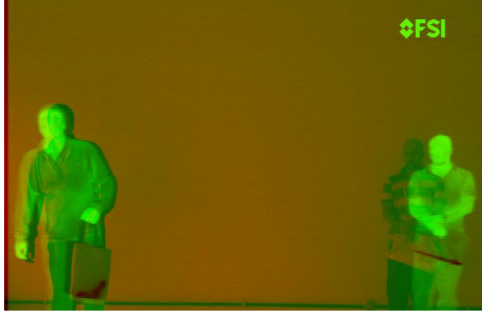
Figure 6.21: Stretching effect caused by the focal length mismatch between the IR and visible-light camera. The visible-light and IR images occupy the red and green channels, respectively, within the depicted RGB pseudo-color image.
