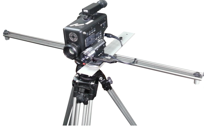
Figure 6.17: Utilized test setup consisting of an IR (left) and visible-light camera (right) mounted side-by-side.
