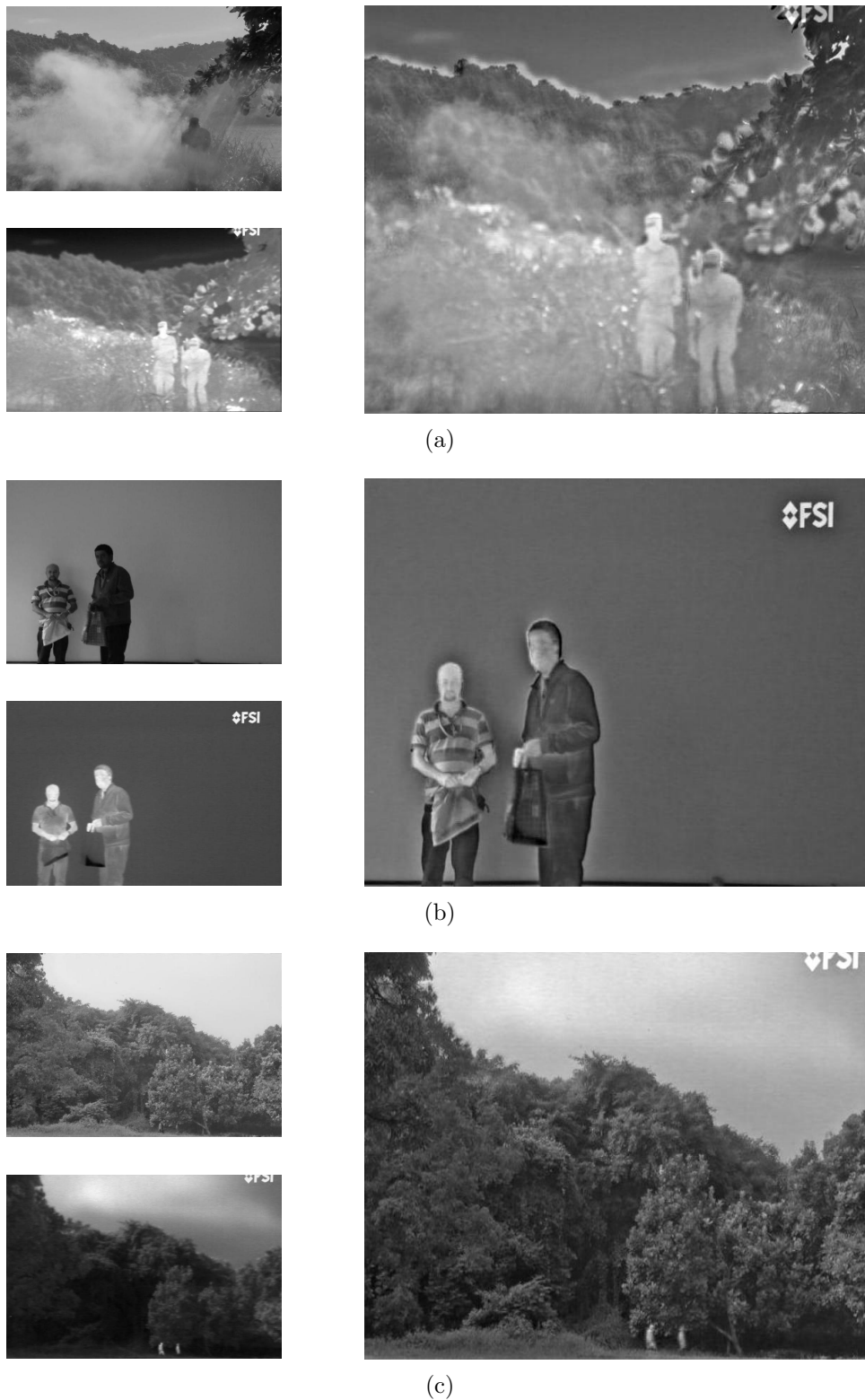
Figure 6.22: Fusion results for selected IR/visible-light image pairs from the (a) “Forte São João 4”, (b) “IME Laboratório de Maquinas 2” and (c) “IPqM Campo 2” video sequence. The fused images are depicted in the right column whereas the visible-light (top) and IR images (bottom) are located in the left column.
