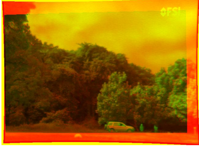
Figure 6.12: Result of image rectification for a sample IR/visible-light image pair. For visualization purposes, the two images were overlaid on top of each other and occupy the red (visible-light) and green (IR) channel within the depicted RGB pseudo-color image.
