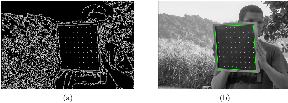
Figure 6.5: Results of the calibration board detection for the visible-light calibration image of Fig. 6.4(a). (a) Segmentation result of the marker-controlled watershed transformation. (b) Detected calibration board after application of the Hough transform.
