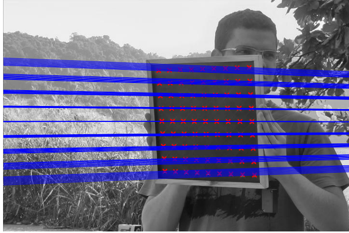
Figure 6.11: Result of stereo calibration when mapping the IR calibration points of Fig. 6.6(b) to the visible-light calibration image of Fig. 6.6(a). Note that due to lens distortion this mapping is no longer linear, resulting in curved epipolar lines.
